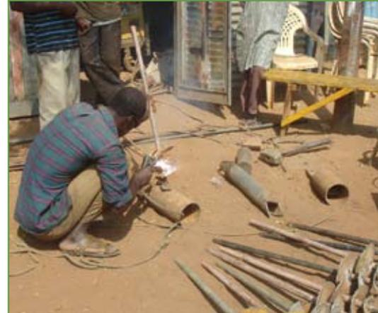
*Construction of Drilling Tools*
