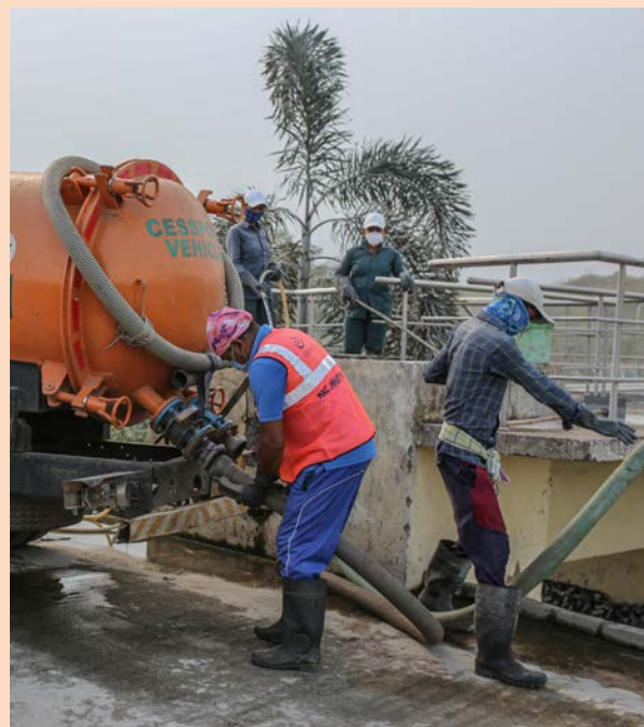
Swachhta Saathi unloads faecal sludge using a Cesspool vehicle inside a Faecal Sludge Treatment Plant (FSTP) at Ganjam District in Odisha.
