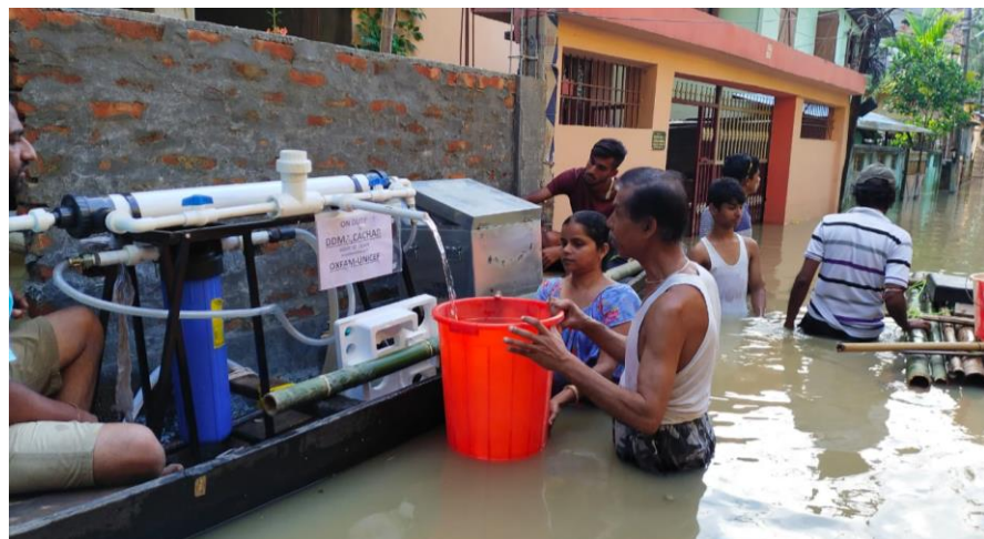
UNICEF supported water treatment unit mounted on a boat providing drinking water to affected areas in Silchar, Cachar
