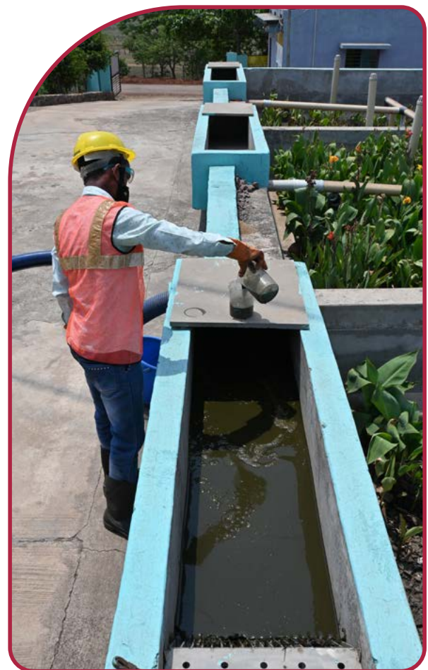
Sanitation worker collecting water sample for treatment
