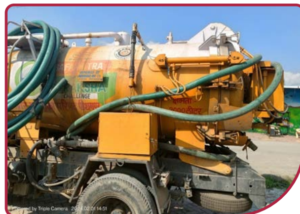
Sludge-collecting vehicle at the FSTP (Faecal Sludge Treatment Plant), Kumhari.
