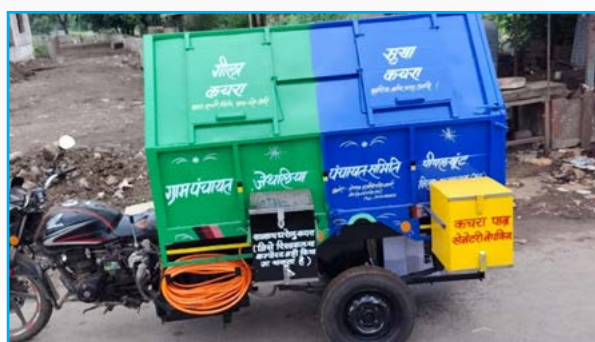
Innovative sanitation vehicle with bifurcation for biodegradable and non-biodegradable waste
