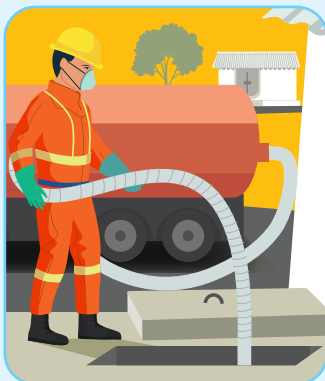
Desludging/emptying of septic tanks/pits
