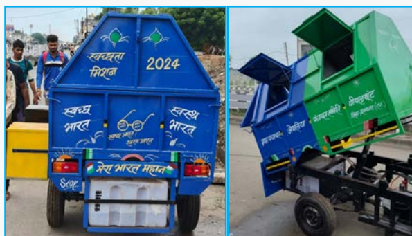
Left - 300-litre water tank fitted in the vehicle for drain cleaning, CSC cleaning, etc. Right - the hydraulic system for emptying waste showing separate chambers for biodegradable and non-biodegradable waste
