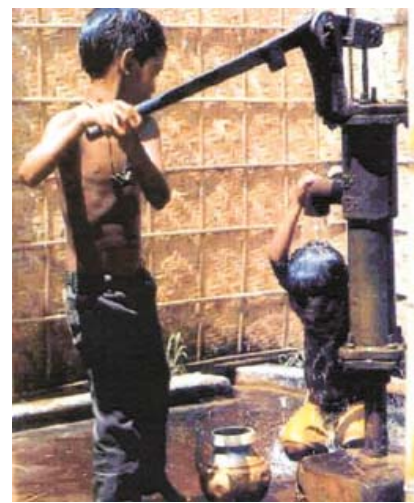
Figure 2: Arsenic-contaminated groundwater in a household tube well with hand pump, Bangladesh
